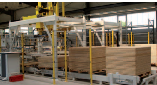
Shown in the foreground are the stacked laminated cores at the beginning of the rotating production line. In the background are the automatically stacked, finished Duroboards.
